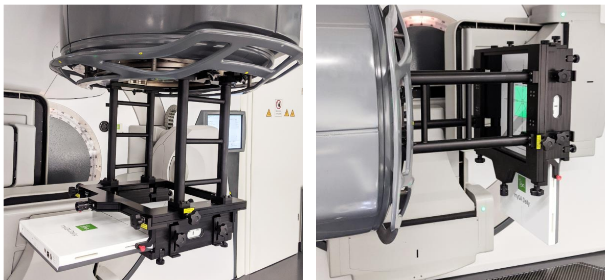
Fig.: Gantry Mount with detector array with gantry at 0° position (left) and at 270° position (right)
